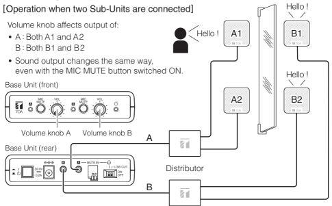
Note: Up to 3 Sub-Units each can be connected to A and B jacks.
